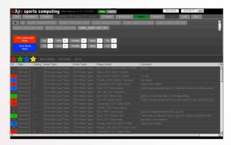
The Dixon Hilite Selector runs on most commonly used NLE's and enables the quick collection of clips to be edited in a highlight package. Bridging the gap between the Loggers and the editors, the Hilite Selector gives the editor immediate access to the logged video via its metadata.
