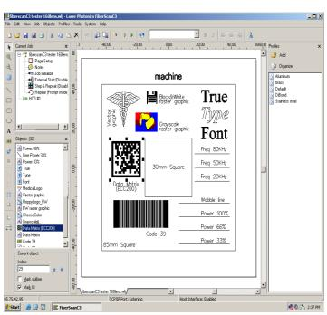
These databases include a materials application system and a fixture database. The materials application system allows a user to define a laser process, give the process a unique name and subsequently link the process to graphic programs. A process can include multiple passes using different values for power, frequency and speed on each laser pass. The database can contain and manage many thousands of different process 'recipes'.
