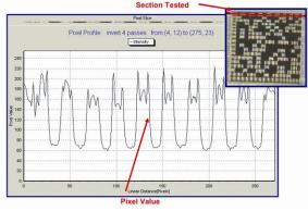
how the MQA<sup>™</sup> software reads the level of pixels in the material marked. The section in red has been analyzed with the MQA<sup>™</sup> software. The high and low pixel values demonstrate the overall contrast of the mark. This procedure can be applied to various different marking processes and types generated by our Fiber Laser marking systems.
