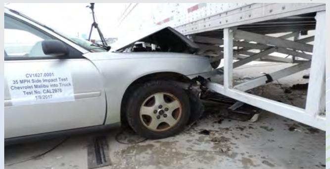
Crash\*\*\* with AngelWing™ Side Underride Protection device
