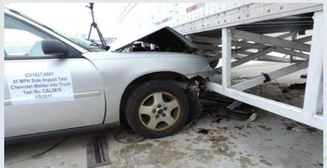
Crash\*\*\* with AngelWing™ Side Underride Protection device
