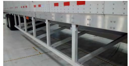
*Full steel frame construction mounts to the existing cross members of the trailer body. Sold in kits, easy to install and fully tested to provide protection up to 35 mph.*
