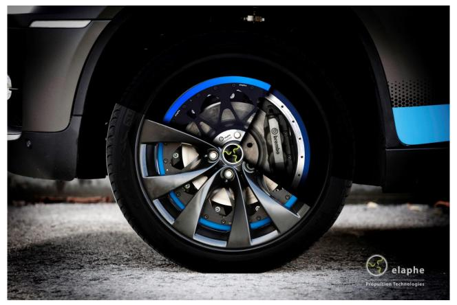
Believed to be the highest-performance in-wheel powered vehicle in the world, the demonstrator is driven by four innovative high-power gearless electric motors (Elaphe™ L1500) mounted inside the rims, enabling the EV to accelerate from 0 to 100 km/h (0–62 mph) in under 4.9 seconds at a weight of 2390 kg (~5300 lbs.).
